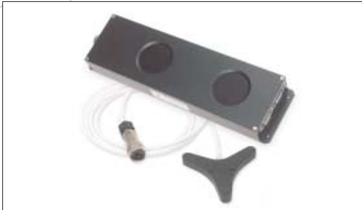
Scanner unit and sensor with cables.
